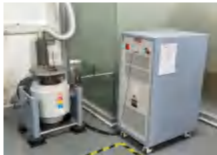
振动系统 正弦扫频、随机扫频 频率、加速度、位移可调 Eletromagnetic Vibration Tester Sine frequency sweep/ Random frequency sweep Frequency/Acceleration/ displacement adjustable
