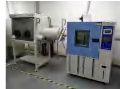
强制内部短路试验机&手套箱 电压实时监控≥100次/s 压力可控可调 Forced internal short circuit test machine &Golve box Real-time monitoring voltage ≥ 100 times per second Voltage can controlled and adjusted
