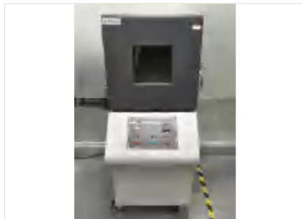
模拟高空低压试验箱 保压≥98% 自动补压 Simulated altitude low pressure test chamber Pressure maitaining≥98% Automatic pressure
